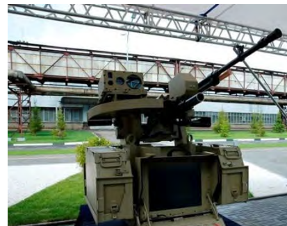
"The Kalashnikov 'combat module' will include 7.62-millimeter machine gun coupled with a camera attached to a computer system. According to TASS, the module uses 'neural network technologies that enable it to identify targets and make decisions'."
